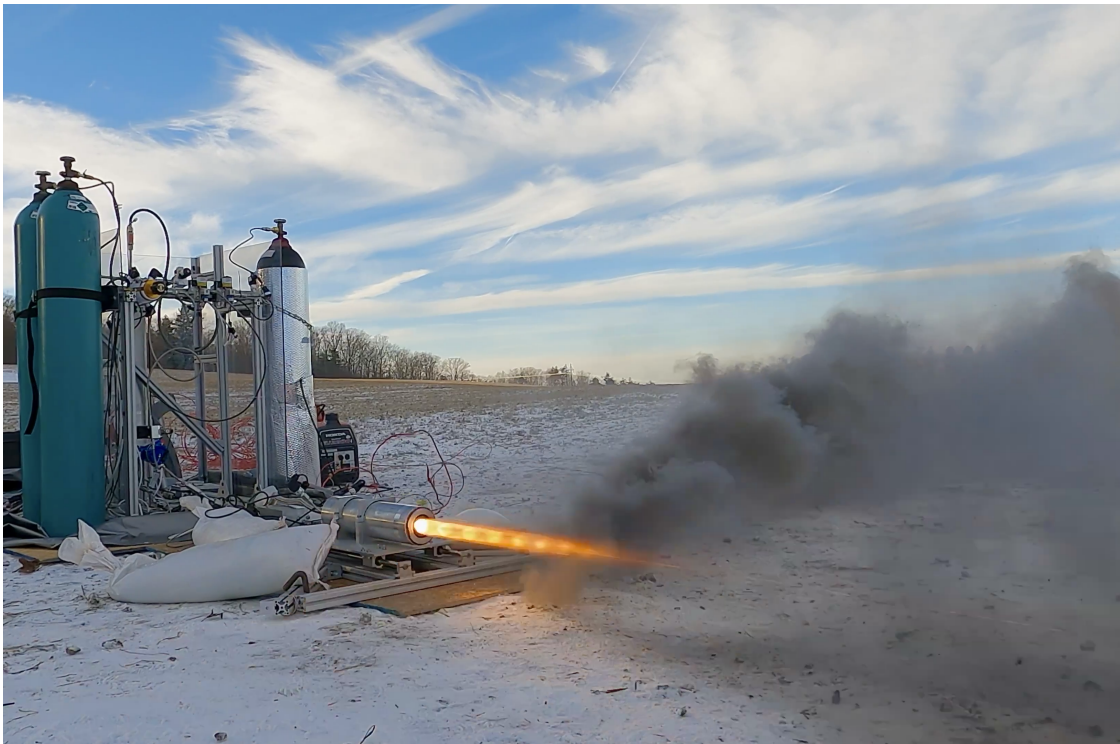
Figure 2: 250 lbf Hybrid Engine Test
