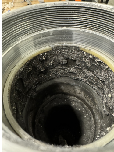
Figure 4: Pre-Combustor Burn Through
