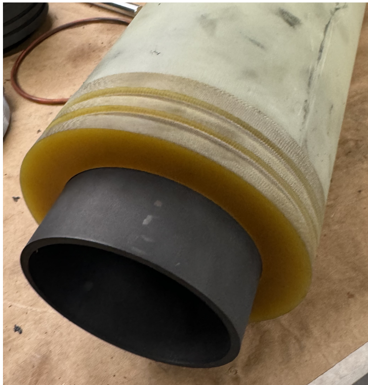
Figure 8: Fiberglass Nozzle Carrier and Liner
