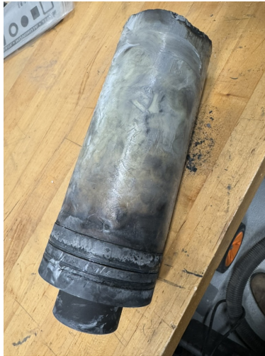
Figure 7: Post-Combustor Burn Through
