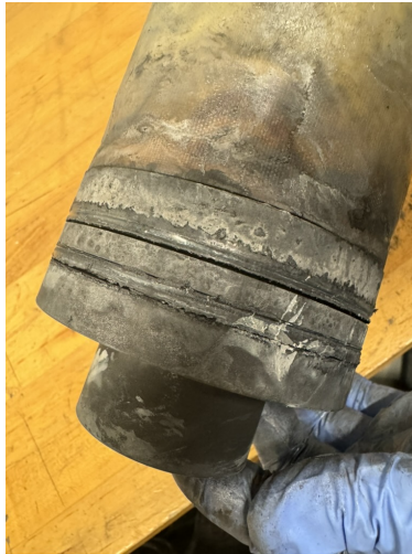
Figure 5: Nozzle O-Ring degradation
