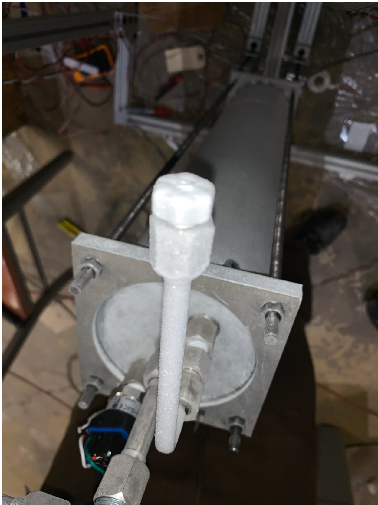
Figure 9: Ice accumulation on dip tube outlet
